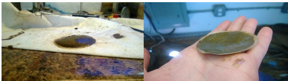
HTHP filter cake at 250 °F before and after washing well #3
